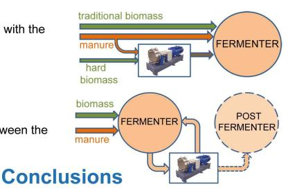
Ricirculation on the digester or between the digesters
